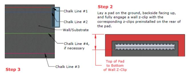
To measure for the upper z-clip placement, take a measurement from the top of the pad to the lower edge of the wall z-clip inserted during Step #2. This is the distance you will measure down from the horizontal line marked during Step #1. Snap a second horizontal chalk line on the wall at this elevation. (Chalk Line #2)
