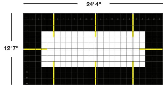
We recommend Expansion Joint strips be placed every 5' to 7' feet depending on exposure to direct sunlight. Length of the strip is dependent upon the sunlight exposure to that section. A minimum of 3' to 4' feet deep is recommended.
