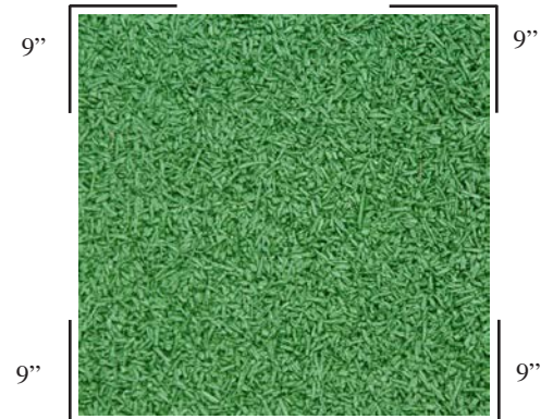
Tile to Tile CX-948 Placement 1/4" wide bead 9" in from all 4 corners
