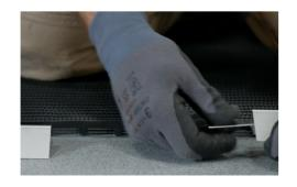
Miter the corners at a 45-degree angle with a power saw. Join using the right angle inserts.
