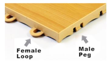
**Step 2** Start by laying your first panel in any corner (male edges required) or garage opening (female edges required) roughly ¼ to 1" from the wall. The loops should be pointed in the direction you want to add panels:
