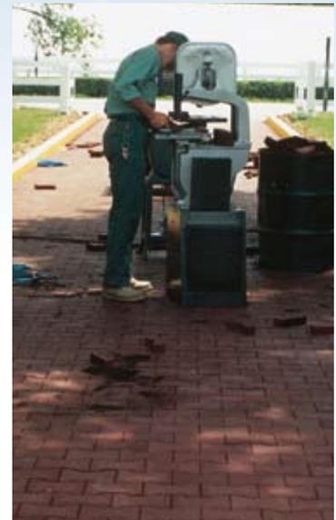
Pavesafe can easily be cut with a heavy duty band saw or a break-off-blade utility knife, pending the size of the project.
