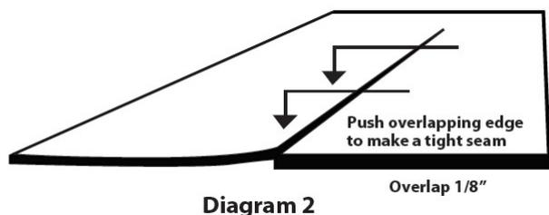
15. It may be necessary to trim the edge of the second lineal drop if the rolls do not extend the length or width of the room. Rolls laid end to end with a variance in roll width greater than 1/4" could result in peaked seams.
