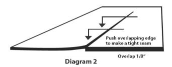
NOTE: Over compressing the seam will result in bond failure at the seam edge.
