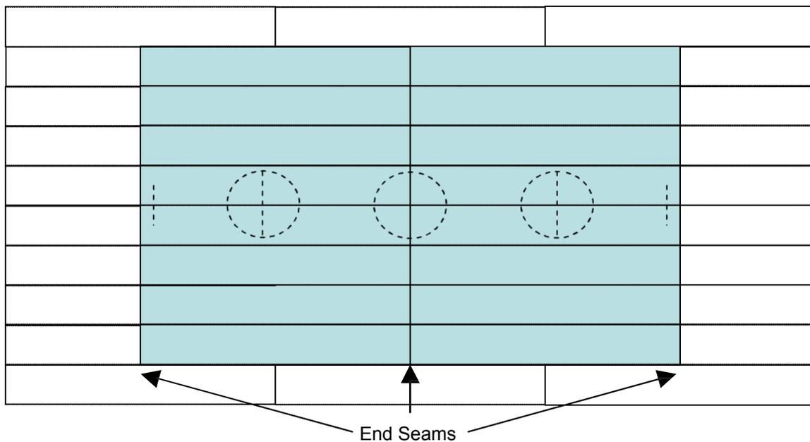
6.6 Seam Cutting: The edges shall be trimmed using a straight edge and a sharp knife or an edge trimmer designed to trim the factory edge of sheet vinyl flooring. Do not use factory edges at seams. Sheets shall be fitted and laid precisely next to each other, without any gaps. Do not pressure fit or allow the seams to peak.
